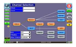
PDH/DSn client can be multiplexed and mapped into SDH/ SONET, which in turn can be mapped and multiplexed into OTN using bit-synchronous or asynchronous modes. In synchronous mode the Optical Payload Unit (OPU) clock is derived from the mapped client signal while in asynchronous the OPU clock is independent.
