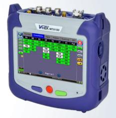
The MTX150 is a fully-integrated and self-contained multi-service test solution for OTN, SDH, SONET, PDH, DSn, Ethernet, SyncE, Mobile Backhaul, and Fibre Channel (SAN). This all-in-one, rugged and ultra-portable field hand-held test set can be configured with interfaces and technologies required by field technicians to install, verify, maintain and troubleshoot Transport, Metro, Access communication links and services, including legacy applications.
