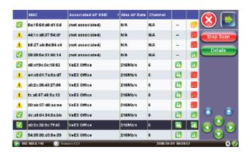
The Air Expert Client scan function monitors all WiFi channels to detect WiFi clients with the SSID they are associated to, as well as non-associated clients (clients not connected to an AP). Network administrators can ensure that the devices are authorized on the network by checking against their MAC address and manufacturer information as well as monitor the client's activity.
