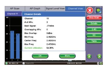
Detailed channel measurements can be sorted by any field including utilization %, number of APs, number of co-channel APs and strongest signal. This information is crucial as technicians need to identify if performance issues are linked to high channel utilization and must quickly decide if reconfiguring the AP to a new channel is advisable.
