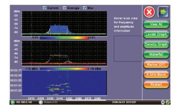
The Air Expert offers a dedicated spectrum analyzer that displays all RF activity - WiFi and non-WiFi interferers - in the 2.4 GHz and 5 GHz bands. The Spectrum Analyzer view allows technicians to visualize interference sources overlapping with the AP under test. The WiFi interference library can also be used to identify interference signatures against a list of known interferers (Cordless phones, Zigbee, Bluetooth, etc.)
